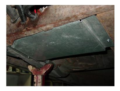
I cut a piece of galvanized sheet metal to fit over the pump and secured it with two screws for protection against debris. My grommet selection did not have the proper size for the new holes I drilled so I used some vacuum line slit lengthwise to line the holes where the hose laid against them (upper left).
