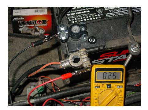
Over the years I have found a couple of batteries that must have had an internal draw of some kind, A quick battery change cured the draw so if you don't find the problem quickly, try swapping batteries before going to the following procedure.
