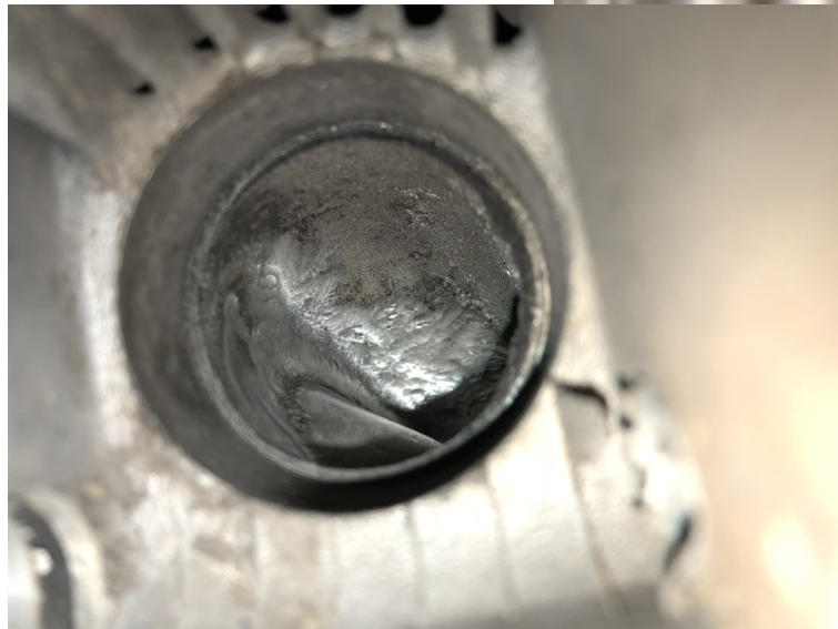
Big Casting Bump in exhaust port removed
