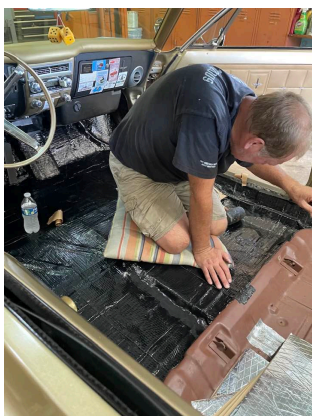
Joe Nels replacing underlayment
